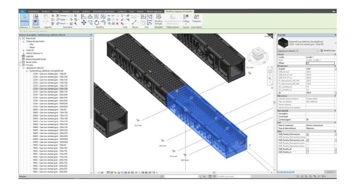
4. Once the object has been positioned, it is possible to manage the instance parameters (linked to the individual objects created in the model and not to the type of objects) such as the presence of end closing bulkheads using the parameters from the properties dialog.
