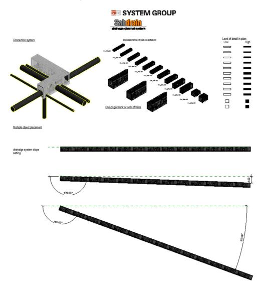
The BIM object "SABDRAIN" is intended, to be added to the project, as a loadable <family>. The object is presented in a Revit .rte template file from which it is easy to extract the object in .rfa format.
