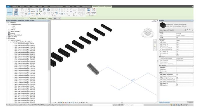
3. Now it will be sufficient to click anywhere in the project space to place the object. For precise positioning it is necessary to click on one end of the channel (marked with a blue dot) and place it at the end of another channel.
