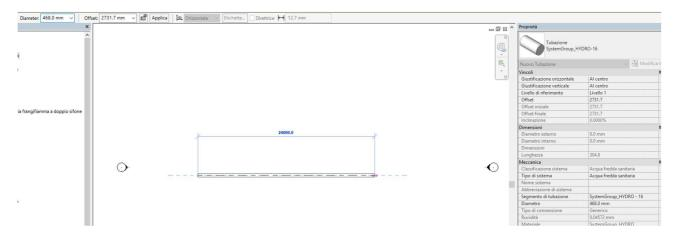
4. It will be possible to change the diameter of the pipe according to the "SystemGroup Magnum" sizes provided by the manufacturer by clicking on Diameter and scrolling the drop-down menu.
