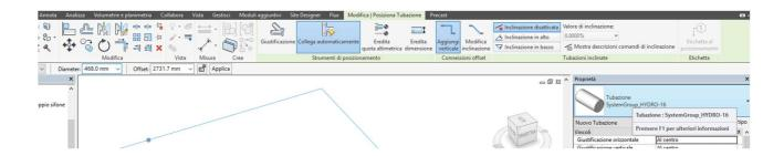
3. At this point it will be possible to draw the pipe assigning with the first left mouse click the starting point and with the second click the end point.
