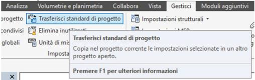
5. When the new window is opened, click <Deselect all> and check only the <Piping> entry, in this way the system family contained in the <System Group> template will be transferred to the project in use
