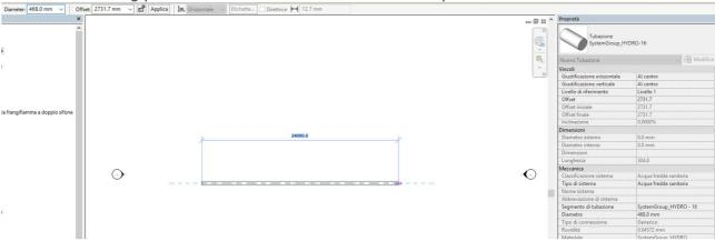
4. It will be possible to change the diameter of the pipe according to the "SystemGroup Hydro 16" sizes provided by the manufacturer by clicking on Diameter and scrolling the drop-down menu.
